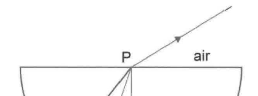
The students vary the position of O to obtain data to determine the refractive index of the glass. They use a protractor to collect values for the angles of incidence  $\theta_i$  and refraction  $\theta_r$  at P and record them on a table.
