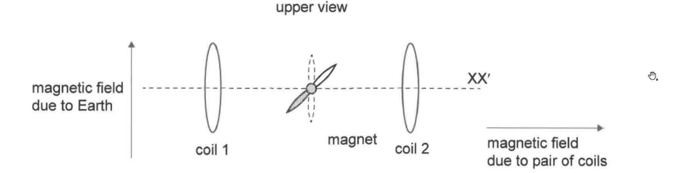
The magnet comes to rest when it makes an angle of 24° to XX'.
